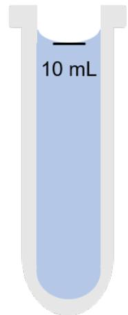
6. The blank is a test tube filled with the sample water, but no reagents. The photometer uses this as a background to compare to your test sample colour.
